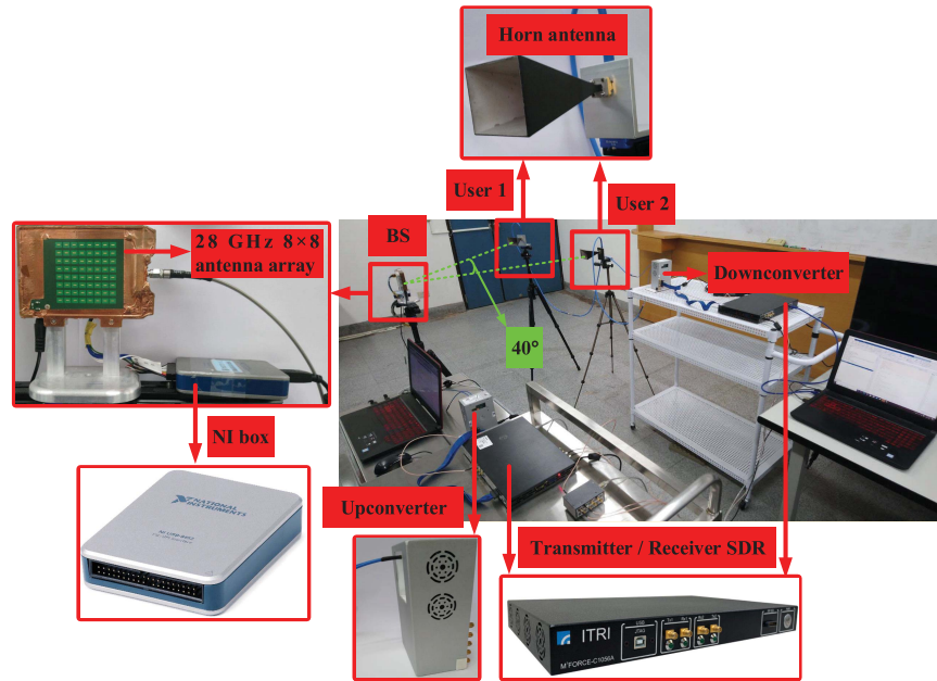
Fig. 11. A photo of the implemented mmWave 28 GHz hardware platform.
